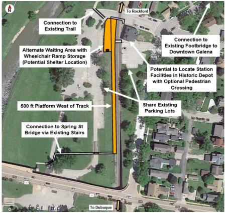
Figure 6: Galena Station conceptual layout
